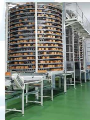
Above Pictures Are PT. Ridar Esindo's Spiral Conveyors That We Manufactured For The Largest Bread Company In Indonesia
